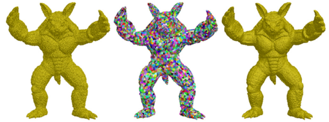
Fig. 7. Clustering-based simplification. From left to right: input mesh (172,962 vertices), clustering result (46,406 clusters), and downsampled mesh (46,406 vertices). Each cluster is rendered with a random color. Please note that, shape features are faithfully retained even under high noise rate.
