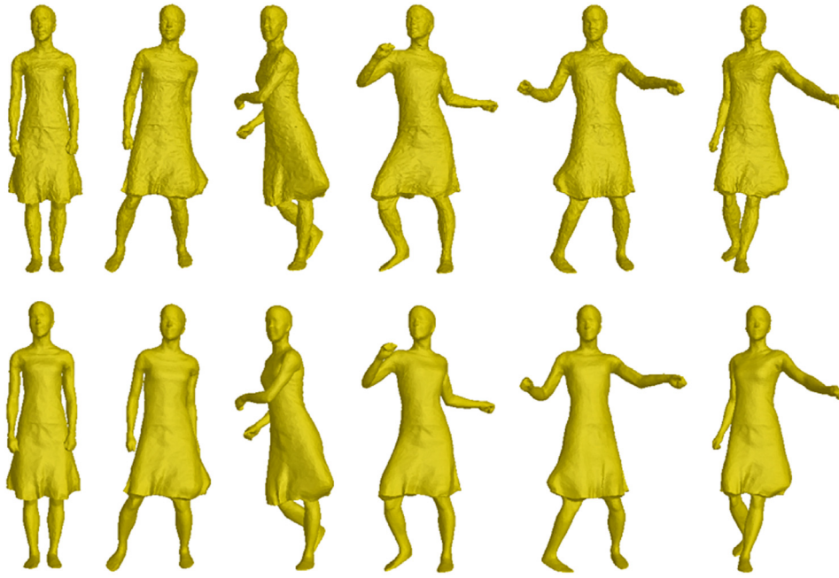
Fig. 14. Denoising result on a swing sequence. From top to bottom: noisy sequence, and our result. This sequence has 150 frames, and each frame has 9971 vertices. Here only six key frames are shown (due to space limitation).
