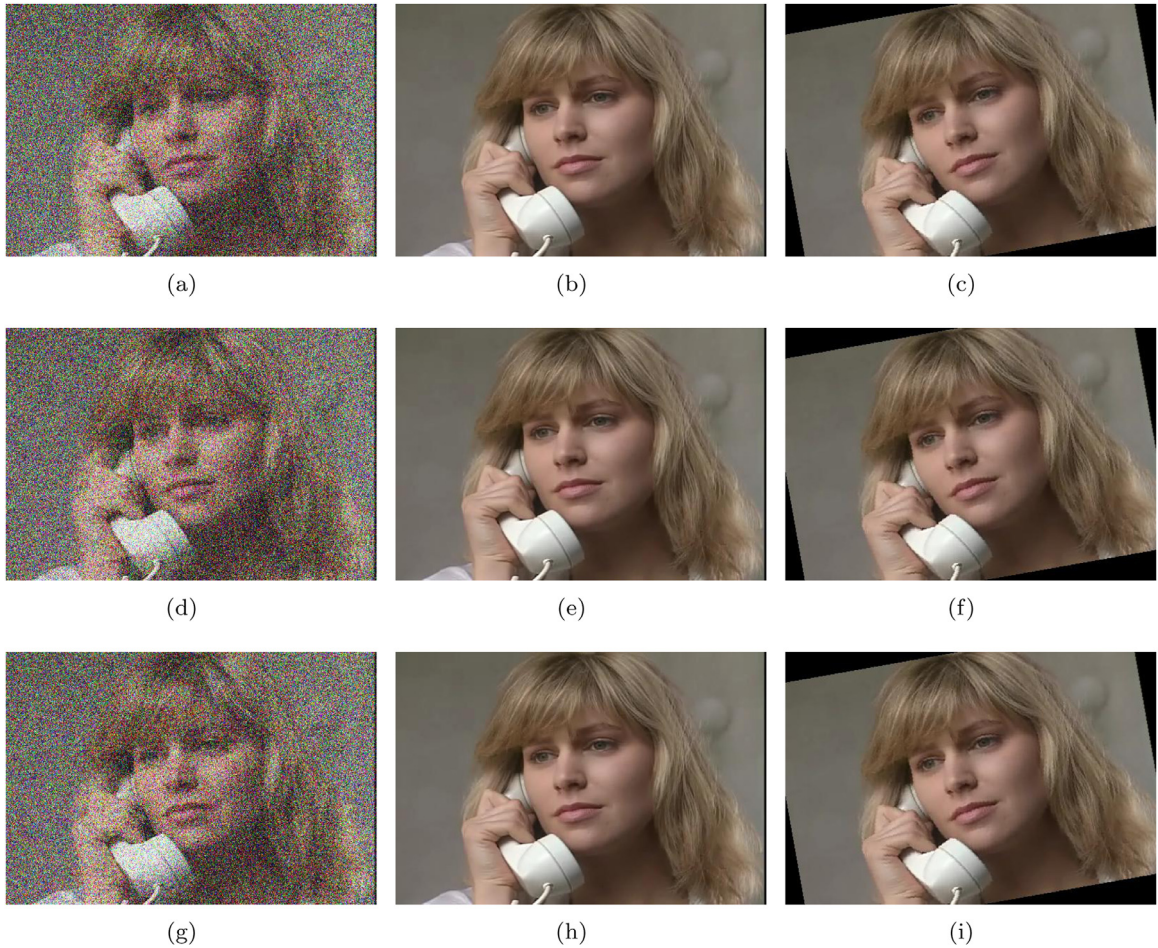
Fig. 16. (a)–(c) are the 300th frame in the watermarked video based on [13] under Gaussian noise, frame averaging and rotation, respectively. (d)–(f) and (g)–(i) are the frames based on [33] and our work, respectively.
