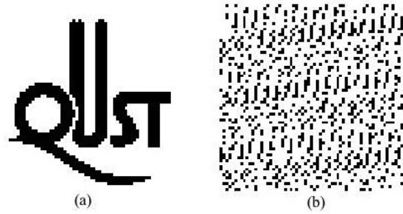
Fig. 5. Watermark encryption with Arnold transformation, (a) original watermark, and (b) encrypted watermark.
