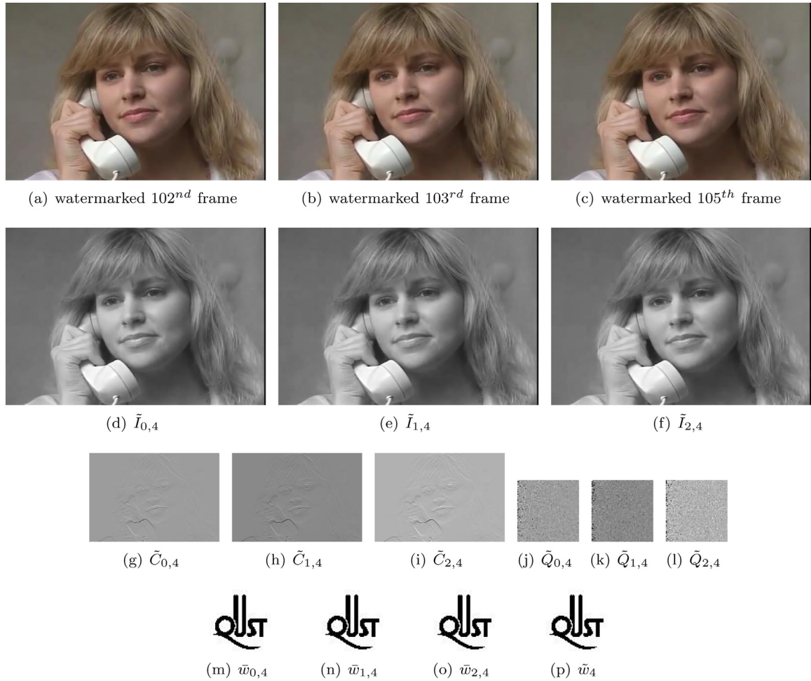
Fig. 12. Watermarked key frames of the 4th scene from suzie.avi to be tested, R components \tilde{I}_{0,4}, \tilde{I}_{1,4} and \tilde{I}_{2,4} , LH wavelet component coefficients \tilde{C}_{0,4}, \tilde{C}_{1,4} and \tilde{C}_{2,4} , target wavelet coefficients \tilde{Q}_{0,4}, \tilde{Q}_{1,4} and \tilde{Q}_{2,4} , extracted watermarks \tilde{w}_{0,4}, \tilde{w}_{1,4} and \tilde{w}_{2,4} from key frames, and the extracted watermark \tilde{w}_4 obtained by combining \tilde{w}_{0,4}, \tilde{w}_{1,4} and \tilde{w}_{2,4} using (19).
